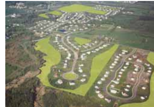
Image showing no interconnectivity between "conservation subdivision" green areas or streets. Natural corridors and land set aside for open space should create networks. An opportunity for combining pedestrian and natural resource connectivity within the village.
